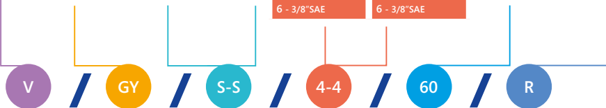
Series GY flexible hose with valve, connections straight-straight, 1/4" x 1/4", 1500 mm, red
